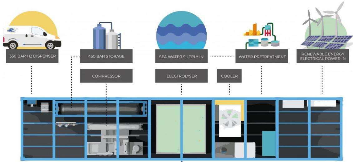
This diagram needs to be read from right to left, but we can follow through each section. One of the key aspects of the SEAFUEL project is that it has been looking at the ability to use sea water for electrolysis. The installation here includes a sea water treatment plant that treats and desalinates the water. As previously mentioned, the water treatment system takes the process seawater and makes it suitable for use in the electrolyser.
